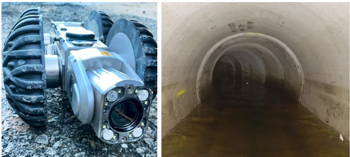
Figure 2: Example of “pipeline crawler” used for drainage pipe CCTV inspections (left) and CCTV footage (right). Photos courtesy of VAPAR, July 2024.
